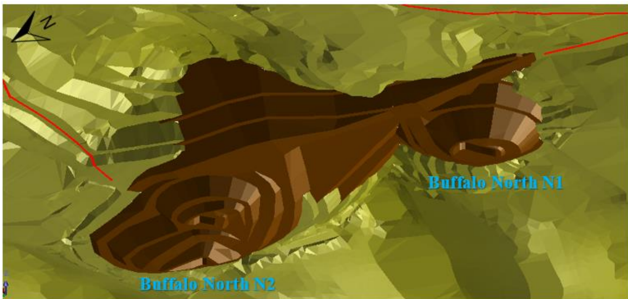
Figure 16.13 Buffalo Reef North pit designs asymmetric view
