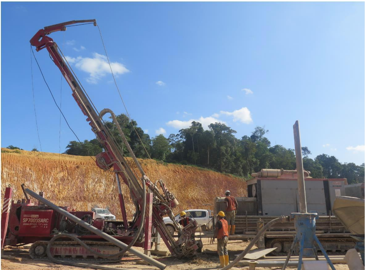
Figure 10.3 RC drilling by contractor at Buffalo Reef (photo taken during 2016 site visit)
