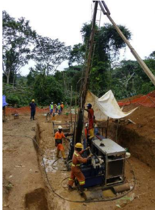
Figure 31. A Discovery 2, helicopter-portable diamond core rig at Ngoy (Source: Regal).
