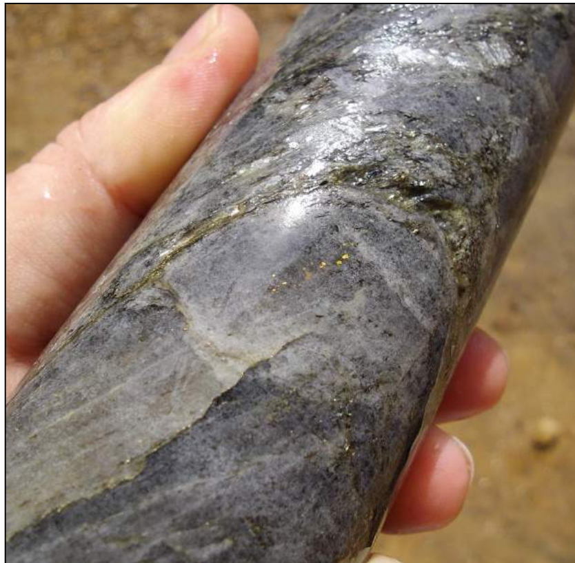
Figure 11. Visible gold in drill hole NGODD004 (55.50 m) hosted within silicified gneiss.
