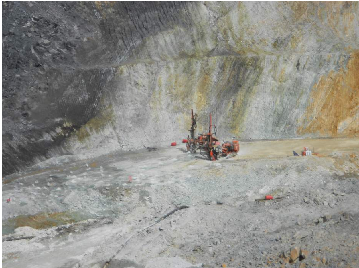
Figure 16.1.2 Selinsing pit bench drilling.
