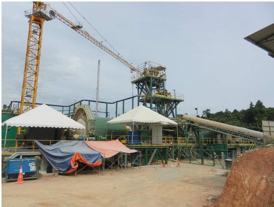
Figure 17.1.2 Primary and secondary ball mills with Knelson Concentrator at Selinsing Mine (June, 2012).
