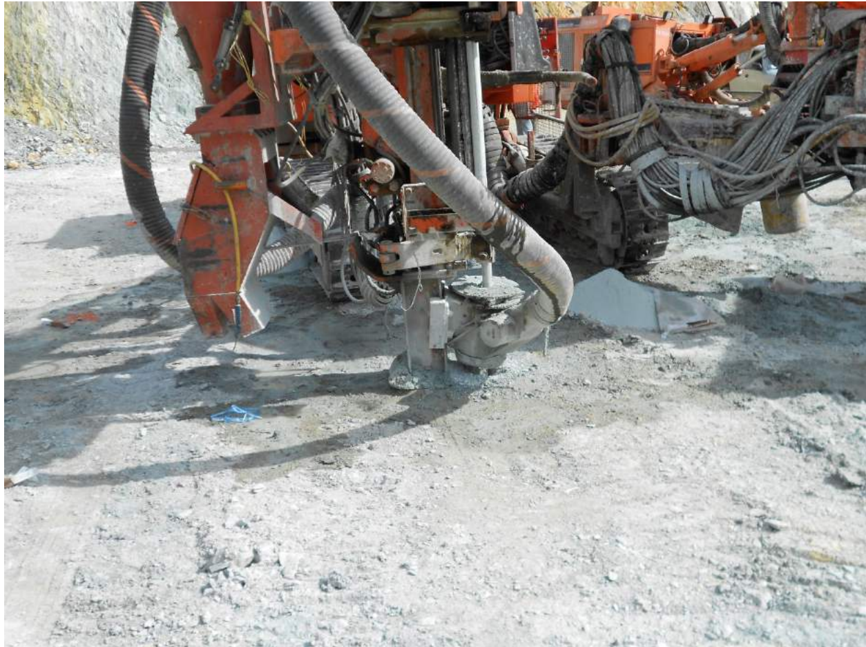
Figure 16.1.3 Automatic sample collector on blast hole drill.
