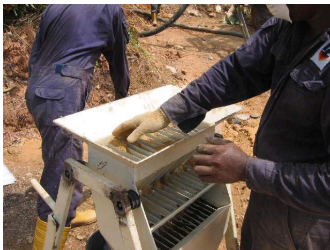
Figure 12.5 Pushing material through the splitter
