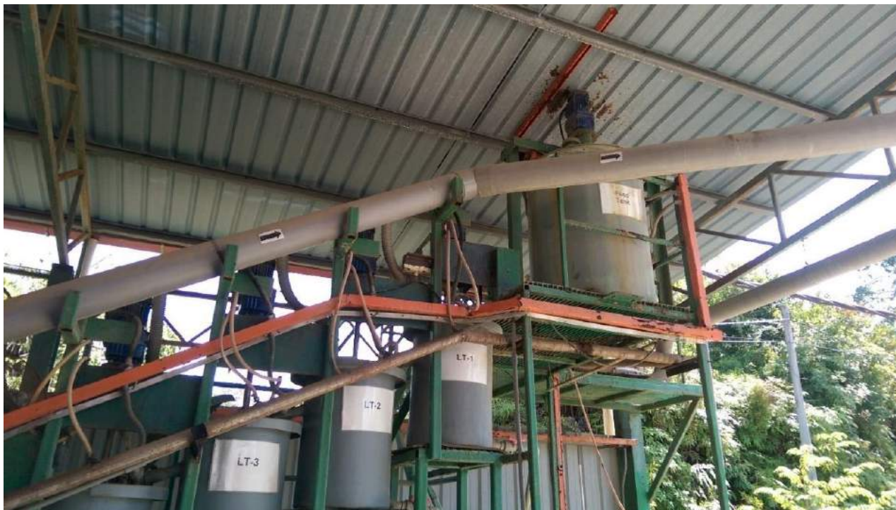
Figure 13.3 Acid leaching pilot plant as employed for testing the Intec Process
