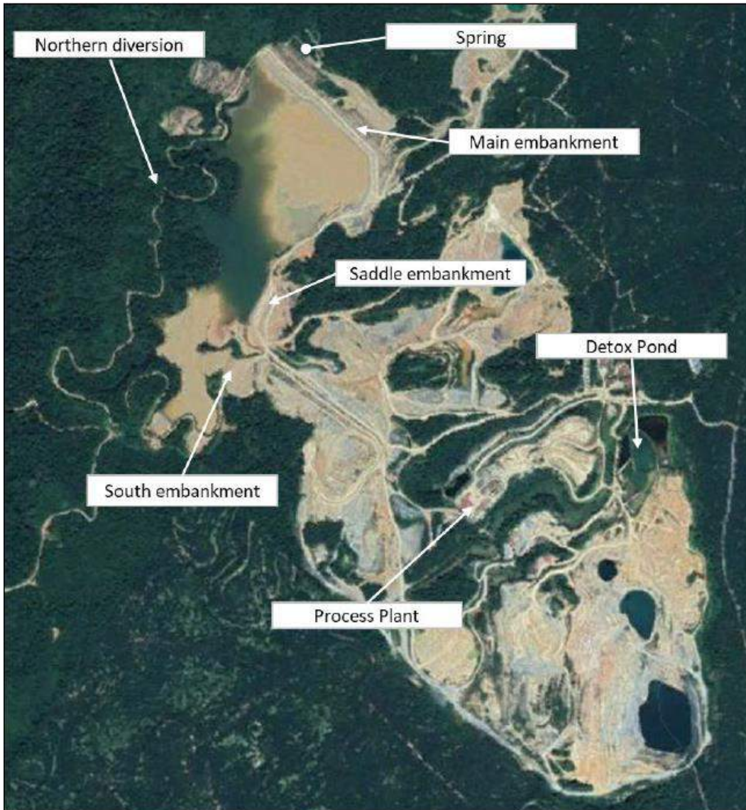
Figure 20.1 Site layout showing TSF location
