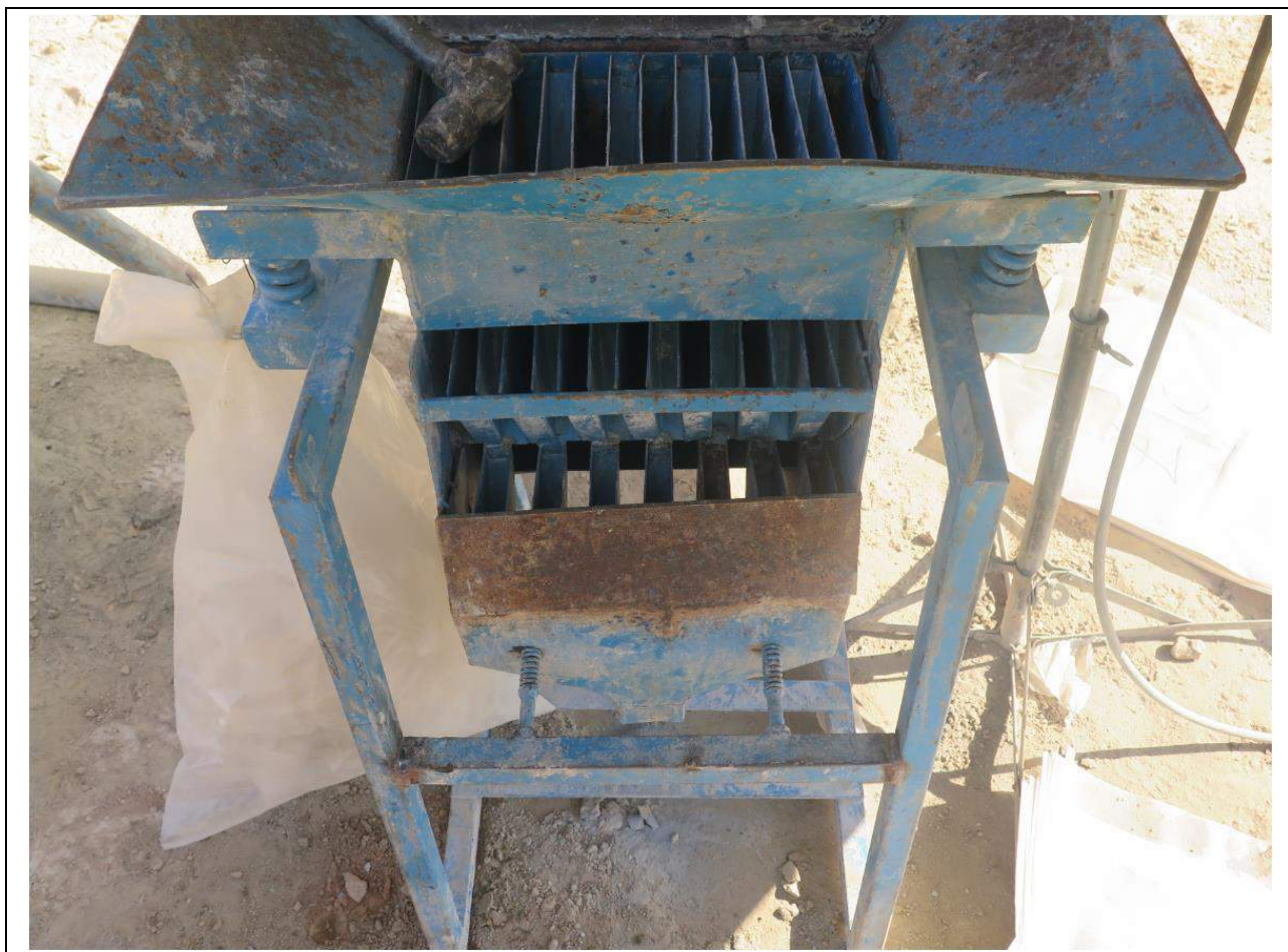
Figure 10.2 Three-tiered riffle splitter (photo taken during 2016 Snowden site visit)
