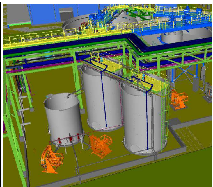
Figure 17.13 pH adjustment tank 1 and 2
