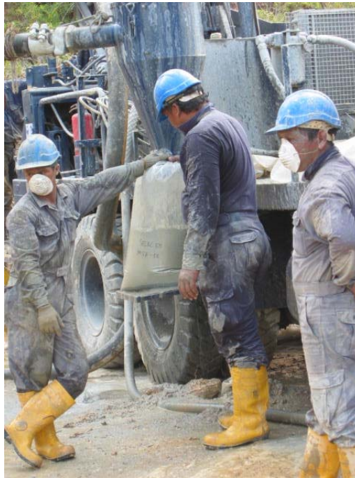
Figure 12.7 Collecting wet sample off cyclone
