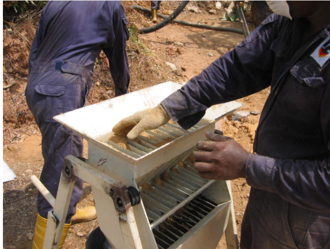
Figure 12.5 Pushing material through the splitter
